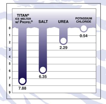
\* Ice melting comparisons measured in milliliters using the testing method set up by the Strategic Highway Research Program H-205.1. Ice melters were tested at 15°F for 20 minutes.
